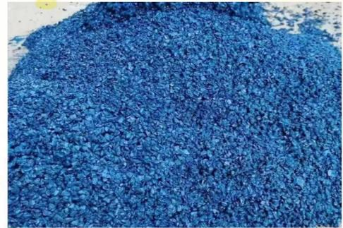
Hot-mix coloured Asphalt Mixture Materials
